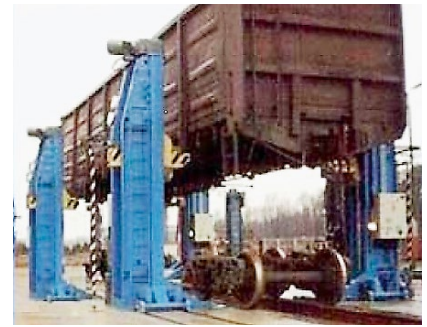
Fig. 1. Kutruuff type screw jacks. Source: Catalogue of equipment and measuring instruments. MTL ASCO RAIL Sp. z o.o. (www.ascorail.eu)
